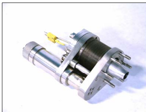
FIG. 6 : 700°C -IR sliding furnace
