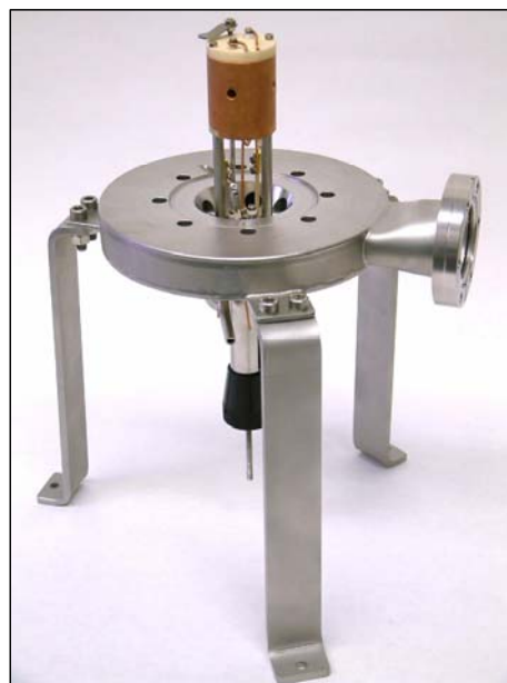
MEG on CF64-CF40 pumping channel
