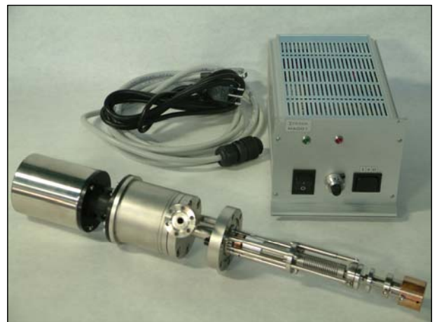
Power supplies and controls for target
