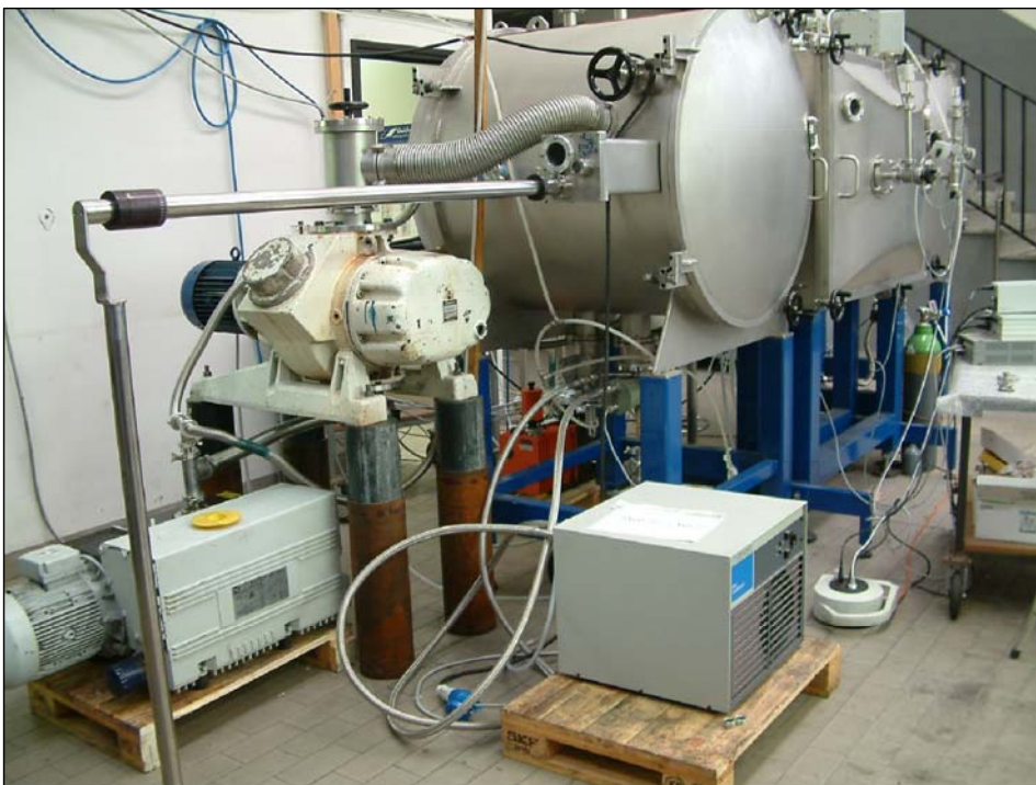
Fig 2 Pumping group of intrduction chamber
