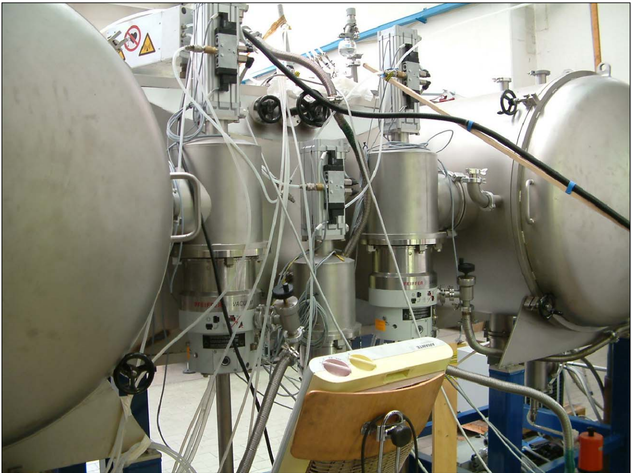
Fig.5 Angle valves and turbo groups
