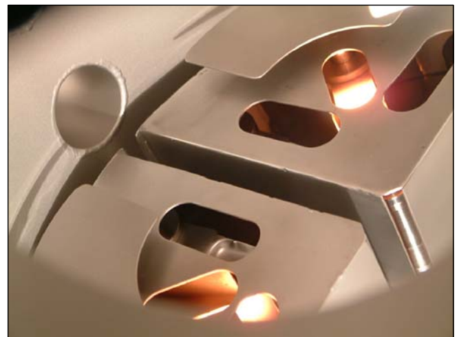
Fig 9 JET300 with two of the six thermal sources during a co-evaporation
